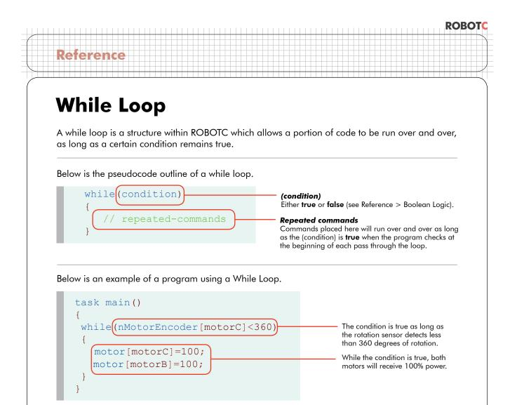
This while loop runs as long as the rotation sensor detects less than 360° of spin. As long the condition remains true, motor A and motor B are told to run at full power. When the condition becomes false, i.e. the rotation sensor detects more than 360° of spin, the loop ends and the robot goes on to the next line of code. In this case, the program ends.
